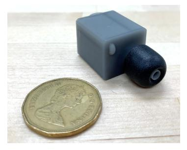
An earplug developed by Doutres and his colleagues has a 3D-printed structure attached to a soft foam plug, which fits into the ear-canal cavity. A Canadian \$1 coin is shown for scale.
