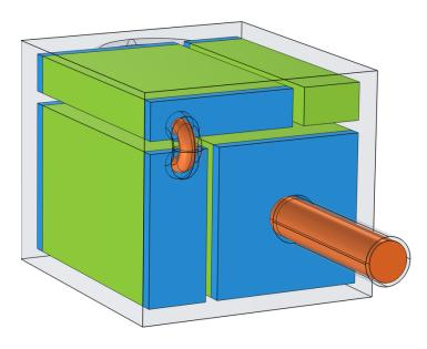
The earplug consists of four foam-filled cuboid cavities (blue and green), connected by hollow, narrow tubes, which together form a resonant structure that traps low-frequency sound waves.
