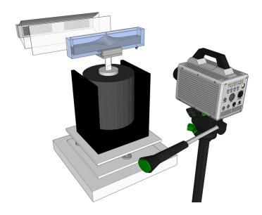
**How the magic is made.** In the experiment, the transparent basin of dyed liquid (blue) is lit from behind by an LED array shining on a diffusive screen. The basin is mounted on an electromagnetic shaker.
