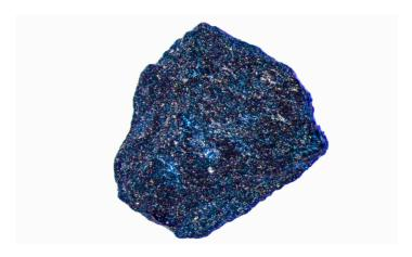
A microscope image of a roughly 1-mm-diameter sample of lutetium hydride. Researchers claim that when doped with nitrogen this material can superconduct at room temperature and near-ambient pressure.
