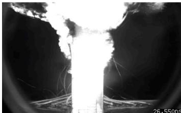
When filled with water, the porous explosive detonates cleanly and completely. (Time shown in nanoseconds.)
