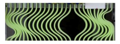
**Pressure to conform.** Green elastic beams are compressed, causing them to bend and push against one another. As compression increases, the beams tend to align. **Credit: A. Guerra** *et al.* [1]
