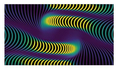
A numerical simulation shows that as the beams become compressed, clumps (where beams press against one another) "annihilate" upon contact with holes (open spaces between beams). Lighter colors indicate regions of higher stored bending energy. In this simulation, the vertical space is fixed, and the beams grow longer with time, whereas in the experiments, the beam lengths are fixed, and the vertical space decreases with time.
