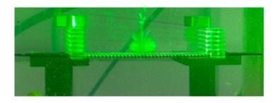
**Calm before the storm.** A vortex ring is illuminated by laser light (required for one of the imaging techniques) just before it strikes the porous structure.
