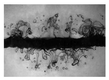
A vortex ring with a high rotation rate (Reynolds number based on circulation: 14,260) effectively removes oil from both the front (top) and back (bottom) surfaces of the porous structure. (Video slowed down by  $133\times$ .)
