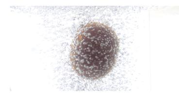
**Scrubbing bubbles.** A tomato is cleaned in a bubble bath. Experiments with a single stream of bubbles directed at a flat, contaminated surface show that the cleaning is maximized when bubbles strike at a specific angle.
