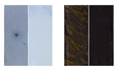
**Maximum cleaning.** "Before" (left photo in each pair) and "after" (right photo in each pair) images of slides initially contaminated with milk and flour proteins (left pair) and bacteria (right pair) and then subjected to six minutes of the bubble treatment at an inclination angle of 20°.
