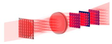
**Thousand points of light.** In the team's setup, a laser beam strikes a microlens array at the left. Optical elements focus the outgoing light into repeating 2D patterns of spots.
