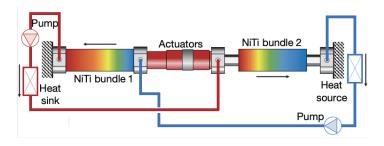
In the system developed by Takeuchi and colleagues, a steel actuator compresses a bundle of NiTi tubes to 700 megapascals (bundle 1). Water is pumped from the cold end of that bundle toward the hot end. At the same time, the actuator unloads a second bundle of NiTi tubes (bundle 2) and water flows from the hot end of that bundle to the cold end.
