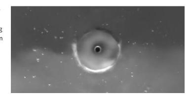
**Video 1:** Disappearance and reappearance of a circular hydraulic jump on a circular plate. The jet has a diameter of 0.9 mm, and the plate has a diameter of 9 cm.
