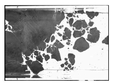
A 20-cm-wide film made of graphite particles floating on water is broken apart by 3-Hz surface waves. In this case they are standing waves, and the breakup begins at one of the antinodes (locations where the wave amplitude is at a maximum).
