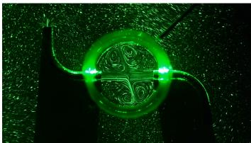
Light-scattering microparticles reveal the flow pattern for the reverse (sucking) mode, showing vortices and complex flow patterns forming inside the central chamber. Here the device is prevented from rotating in order to improve the visualization of the flow.
