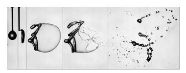
This sequence of images shows what happens when a 2.1-mm water droplet is struck by an airflow. Starting at the left, the initial droplet (time = 0), deformation into a pancake shape (2.8 ms), transformation into a balloon-like structure (6.9 ms), and finally fragmentation into droplets of a variety of different sizes (7.4 ms and 9.5 ms).
