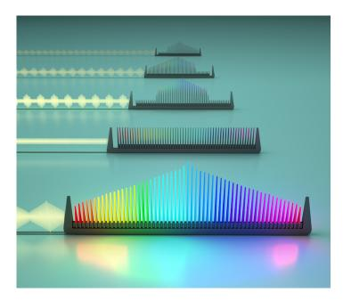
**Comb of light.** A frequency comb consists of a series of short laser pulses that produce light with a comb-like spectrum that depends on the details of the pulse shapes and on their timing. **Credit: Second Bay Studios; Harvard SEAS**
