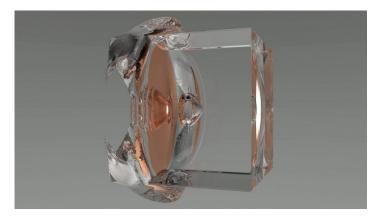
A three-dimensional simulation shows a projectile hitting a cube-shaped target that contains small bubble-like cavities that channel the collision energy to a capsule containing fusion fuel. **Credit: First Light Fusion**
