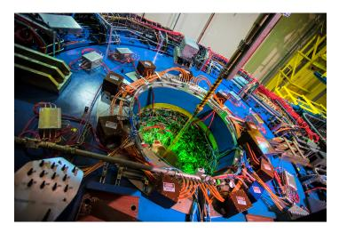
Big detector for big nuclei. The house-sized STAR detector tracks the particles produced by quark-gluon plasmas generated in heavy-ion collisions.
