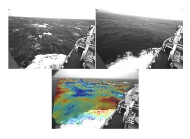
**Before and after.** In a relatively young sea state (top left), winds drive slow moving waves, which grow steeper and often break, causing white caps and seas with rogue waves. In an older state (top right), waves move faster but are less steep, giving calmer seas. The stereo cameras produce a color-coded map (bottom). In this example, the elevation ranges from about one meter below sea level (dark blue) to about one meter above sea level (dark red). **Credit: A. Toffoli et al. [1**]
