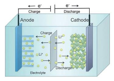
A lithium-ion battery consists of an anode, a cathode, and a liquid electrolyte between them. Lithium ions move toward the anode when the battery charges and then move back to the cathode when it discharges. Electric current flows into and out of the battery through the wire connections at the two electrodes. Credit: P. Roy and S. K. Srivastava [2]; adapted by APS
