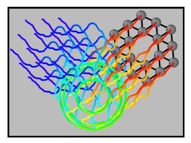
**Ring of activity.** Numerical simulations reveal two distinct kinds of collective behavior for a hexagonal ring of 18 active elements linked together in a rigid triangular lattice. The system can either rotate coherently or translate linearly in any direction. Trajectories are color coded to indicate time, with the earliest times in blue and the latest times in red. (See animation below.)
