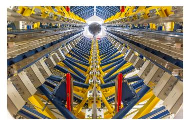
**What goes up.** The Einstein Elevator at Leibniz University Hannover, Germany, creates microgravity conditions by launching experiments upward into a 40-m-tall tower (upward-looking view shown here), providing 4 seconds of freefall during upward and downward motion (**video**).
