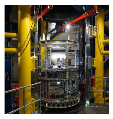
**Freefall.** The INTENTAS experiment (shown here being prepared for operations at the Einstein Elevator) will use the new entanglement-enhanced gravimeter to test the equivalence principle of general relativity.
