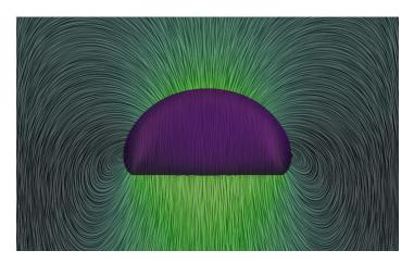
In this computer visualization featured in the traveling gallery, a gas bubble—deformed into an oblate ellipsoidal cap at low speed—rises in a viscous liquid.
