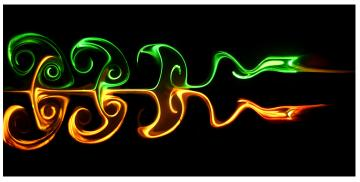
As part of a previous year's submission to the Gallery of Fluid Motion, researchers traced the vortex wake that forms behind synthetic seal whiskers in a water tunnel.
