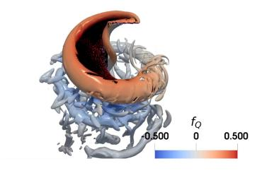
This simulation, featured in the *Spiraling Upwards* exhibit, reveals how da Vinci's aerial screw design is much quieter than the propellers used on modern-day drones.
