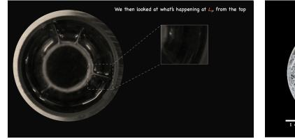
A runny solid flows through an annular channel by turning itself inside out.
