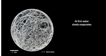
The microstructure of paper and other fiber networks is determined by a balance between capillary forces and fiber stiffness. **Credit: M. L'Estimé/Paris Polytechnic Institute**
