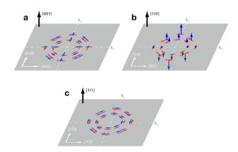
FIG. 1: Schematic depiction of spin-orbit fields as a function of electron crystal momentum in a zincblende quantum well grown along each of three special directions: (a) [001], (b) [110], (c) [111]. The spin-orbit field from the quantum well symmetry is indicated in blue, and the electric-field-induced spin-orbit field is indicated in red. For (c) the two fields have the same momentum-dependent structure. (APS/Alan Stonebraker)
