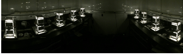
FIG. 1: The digital holographic microscopes used by Leibler and colleagues to study the intrinsic dynamics of a three-species microbial system. Each device observed one replicate of the system, allowing the replicate to be kept under highly controlled external conditions. (Seppe Kuehn and Zak Frentz)
