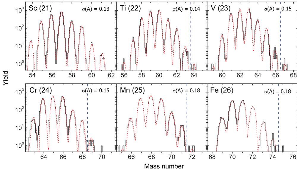
FIG. 3. (Color online) Mass spectra of the elements  $21 \leq Z \leq 26$  that were stopped in the Si telescope during the production runs. The limits of previously observed nuclei are shown by the vertical dashed lines. Standard deviations produced with the Gaussian function at constant width (dashed curves) are given in the panel figures for each element.
