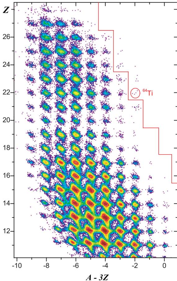
FIG. 2. (Color online) Particle identification plot showing the measured atomic number  $Z$  versus the calculated function  $A - 3Z$  for the nuclei observed in production runs of this work. See text for details. The limit of previously observed nuclei is shown by the solid red line, and the location of  $^{64}\text{Ti}$  is marked.
