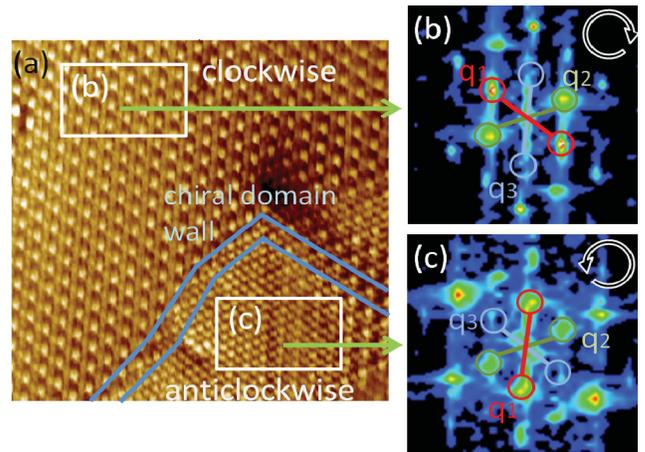
FIG. 2 (color). (a)  $12 \text{ nm} \times 12 \text{ nm}$  STM image and (b),(c) FT of two areas each enclosed with a square in sample B. Sample B was measured at  $V_s = -350 \text{ mV}$  and  $I_t = 0.4 \text{ nA}$  at  $T = 6.3 \text{ K}$ . The blue line is the domain wall between the clockwise phase and the anticlockwise phase.
