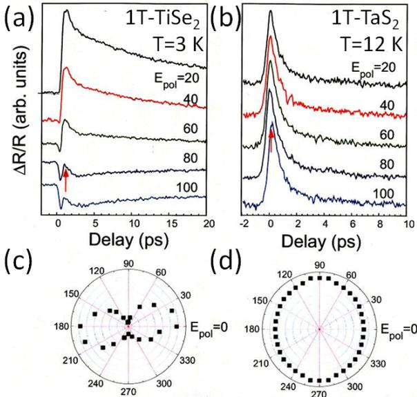
FIG. 3 (color online). Polarization dependence of transient reflectivity variation in  $1T$ -TiSe<sub>2</sub> measured at 3 K (a) and  $1T$ -TaS<sub>2</sub> measured at 12 K (b). The height of each peak is plotted in the (c) and (d) as function of polarization angle  $E_{\text{pol}}$ . The pump pulse wavelength is 1160 nm and the power is 150  $\mu$ W. The probe pulse is 800 nm, 80  $\mu$ W.
