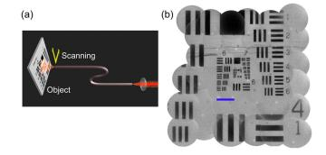
FIG. 3 (color online). Scanning of the fiber end to enlarge the view field. (a) The fiber end at the object side is translated to take images at different parts of the target object. The object images taken at different sites are reconstructed with the same transmission matrix measured at the initial position of the fiber. (b) Reconstructed images are stitched to enlarge the field of view. Scale bar indicates  $100 \ \mu m$ .
