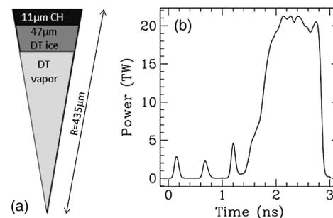
FIG. 2. Low-adiabat ( $\alpha = 2$ ), 24-kJ triple-picket cryogenic OMEGA implosion design (shot 66613) used in 2D DRACO simulations. (a) Target geometry and (b) laser power history. A spherically symmetric simulation of this design without CBET predicts a yield of  $3.4 \times 10^{14}$  neutrons.
