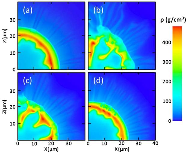
FIG. 3 (color online). Simulated distributions of the density at the peak neutron production for the implosion design shown in Fig. 2. (a) Nominal-size beams,  $R_b/R_t = 1$ ; (b) reduced-size beams,  $R_b/R_t = 0.6$ ; (c) zooming beams from  $R_b/R_t = 1$  to 0.6 at  $t = 0.4$  ns [after the first picket; see Fig. 2(b)]; (d) same zooming beams as in (c), but at  $t = 0.9$  ns (after the second picket).
