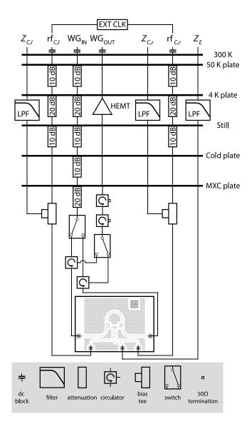
FIG. 5. Measurement setup. Schematic of dilution fridge wiring for measurement. LPF, Low pass filter and MXC, mixing chamber.
