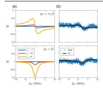
FIG. 9. Extraction of directionality ratio. (a) Theoretical transmission traces for backward excitation of the waveguide, for  $\phi_f = \pi/2$  and  $\phi_f = 0$ . Here, we set  $\Gamma_{1D}^f = 2.5$  MHz,  $\Gamma' = 0$ , and vary  $\Gamma_{1D}^b = 0$ , 25, or 125 kHz. (b) Representative transmission traces show background fluctuations when exciting the qubit from the waveguide in the backward direction.
