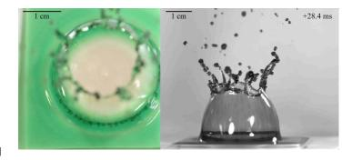
For films over 100  $\mu m$  and with inertial forces dominating over surface tension, the crown forms and eventually collapses in on itself.
