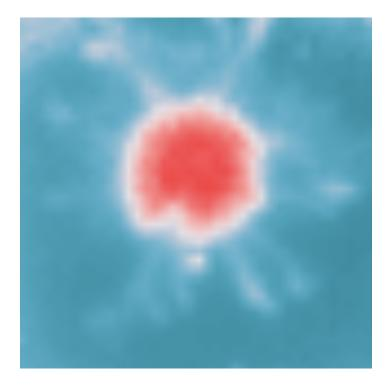
**Hit the spot.** This processed image of the impact point shows the red dye from the drop about 1 second after striking a 103- $\mu$ m-thick water film.
