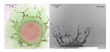
When struck by a falling water drop, the thinnest water films—less than 100  $\mu$ m deep—barely form the "crown" structure before it breaks up into tiny secondary drops.
