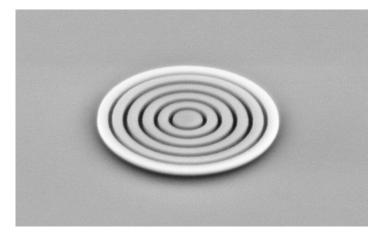
A scanning electron microscope image of the quantum torch. The dartboard-shaped device is roughly 4 μm across. **Credit: L. Rickert/Technical University of Berlin**
